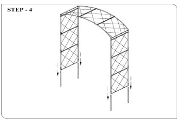
**STEP - 4:** Feet / Rod assembled with Arbor frame and Pushed in grouted as per required depth.
